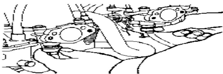
Fig. EF-38 Idle adjust nut
